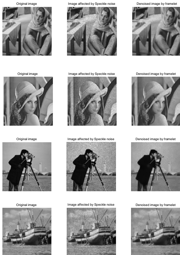
Figure 3 Image Denoising using Framelet (Speckle Noise)
