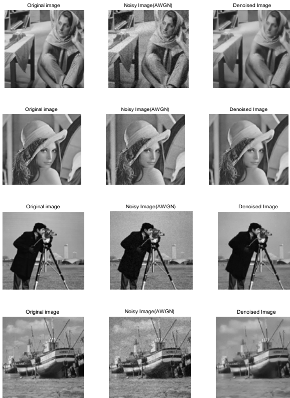
Figure 1 Image Denoising using Framelet (AWGN Noise)
