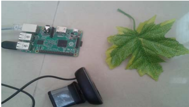
Fig 7: Image capturing system with raspberry pi
